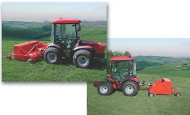
The towed BRUSHING MACHINE is perfect for cleaning Lawn, yard, courtyard and similar areas; the refuse being collected in the rear collector; this basket can be easily overturned and emptied when full, manually or by hydraulic upsetting.
